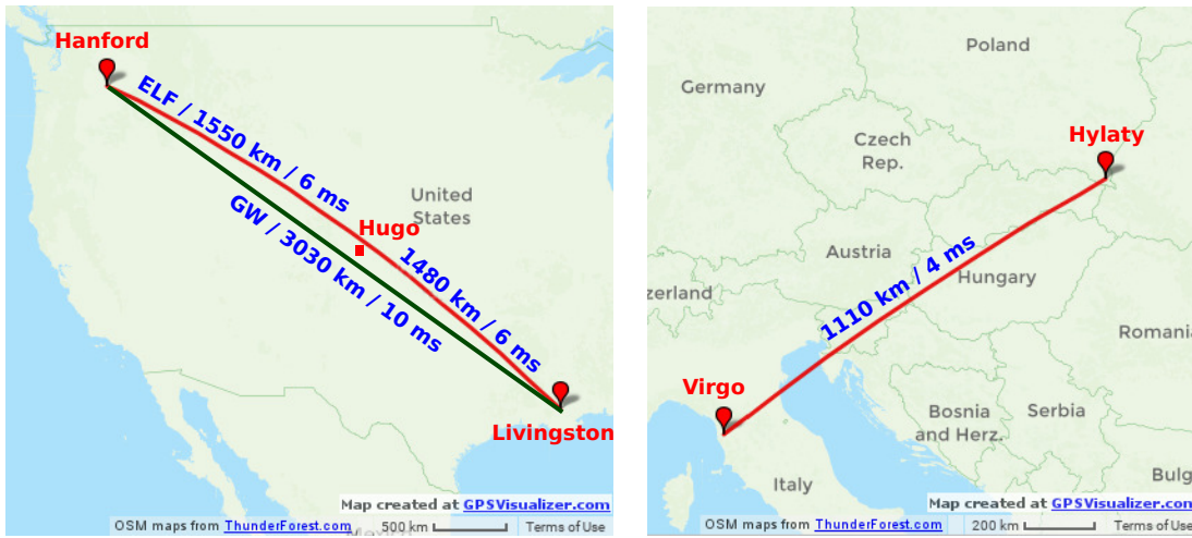
Figure 1. Left: The location of the Hugo magnetometers and the LIGO-Hanford and LIGO-Livingston gravitational-wave detectors, along with the distance separation and the time of propagation for ELF waves. Right: The location of the Hylaty magnetometers and the Virgo gravitational-wave detector, along with the distance separation and the time of propagation for ELF waves.
